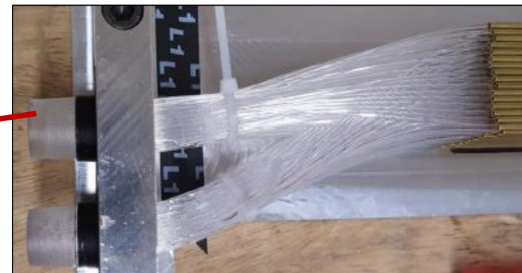
Fiber grouping for PMTs
